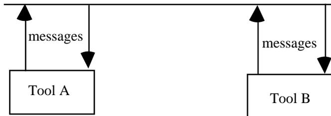
**Figure 3.5 Software tools interacting by passing messages**
