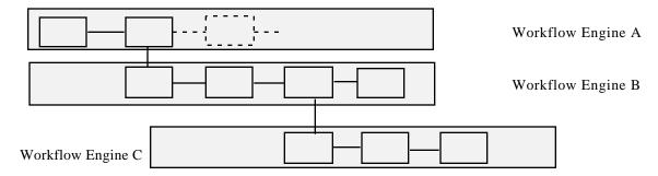
Figure 4.2. main process starts a chained sub-process on another workflow engine which in turn creates a chained sub-process on a third workflow engine
