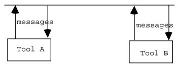
Figure 4-5 Software tools interacting by passing messages
