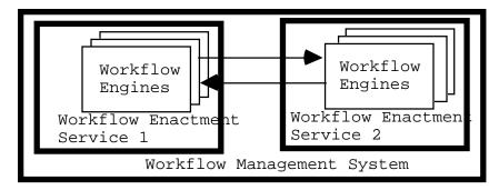
Figure 4-3 Interoperating workflow engines in different enactment services
