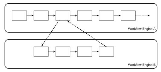
Figure 4-11 The nested sub-process model of interoperability
