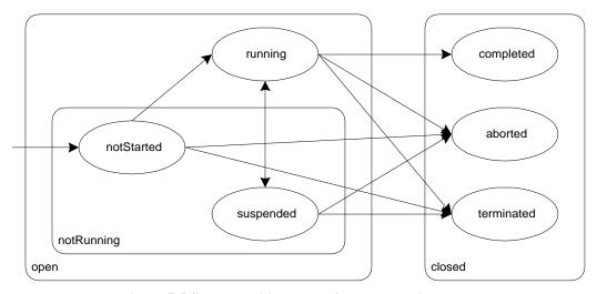
Figure 5-5 State transition model for a process instance
